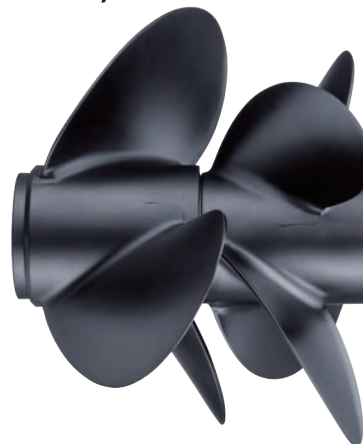
Aluminum / 3 blade front & 4 blade rear / Rubber hub
